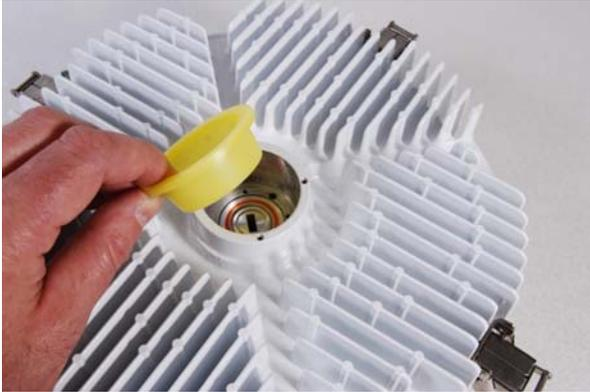
A photograph showing a hand holding a yellow plastic dust cover and pulling it away from the waveguide interface of a white, finned ODU. The interface shows a metal contact point.
