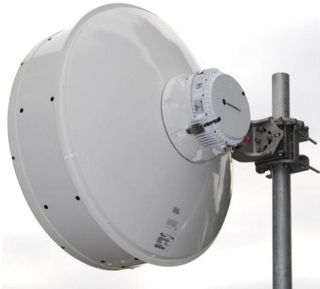
The Motorola direct mount interface (Figure 1-6) provides a reliable and convenient way of mounting the ODU directly to the antenna without the need for additional mounting brackets or waveguides. The ODU fits directly over the antenna's centrally positioned cylindrical transition and is secured in place using the integral spring loaded latches (Figure 1-7). There is no direct mount option for dual polarization configurations.
