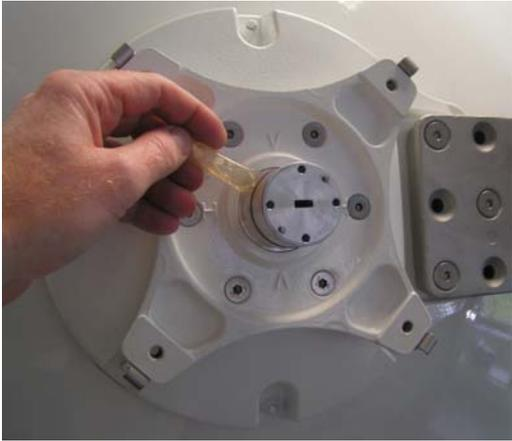
A close-up photograph showing a hand using a small applicator to apply a yellowish substance (silicone grease) to the O-ring of the antenna transition. The transition is white plastic with a central metal waveguide.</div>
